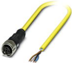
Sensor/Actuator cable, 4-position, PVC, Yellow RAL 1021, Free cable end, on Socket straight M12-SPEEDCON, A-coded, Cable length: 2 m
